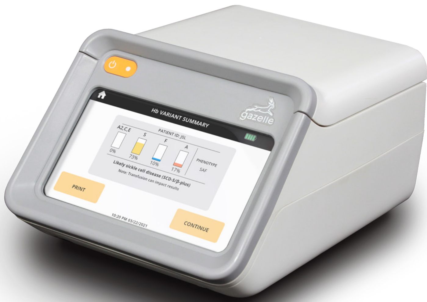
FIGURE 1: Gazelle uses a miniaturized version of the gold standard test: electrophoresis. When a disposable cartridge containing a lysed blood sample is inserted into the reader, a charge is applied to separate the haemoglobin types according to their charge. In 8 minutes, the algorithm determines the haemoglobin types and percentages, and makes the interpretation (normal, trait, disease).
