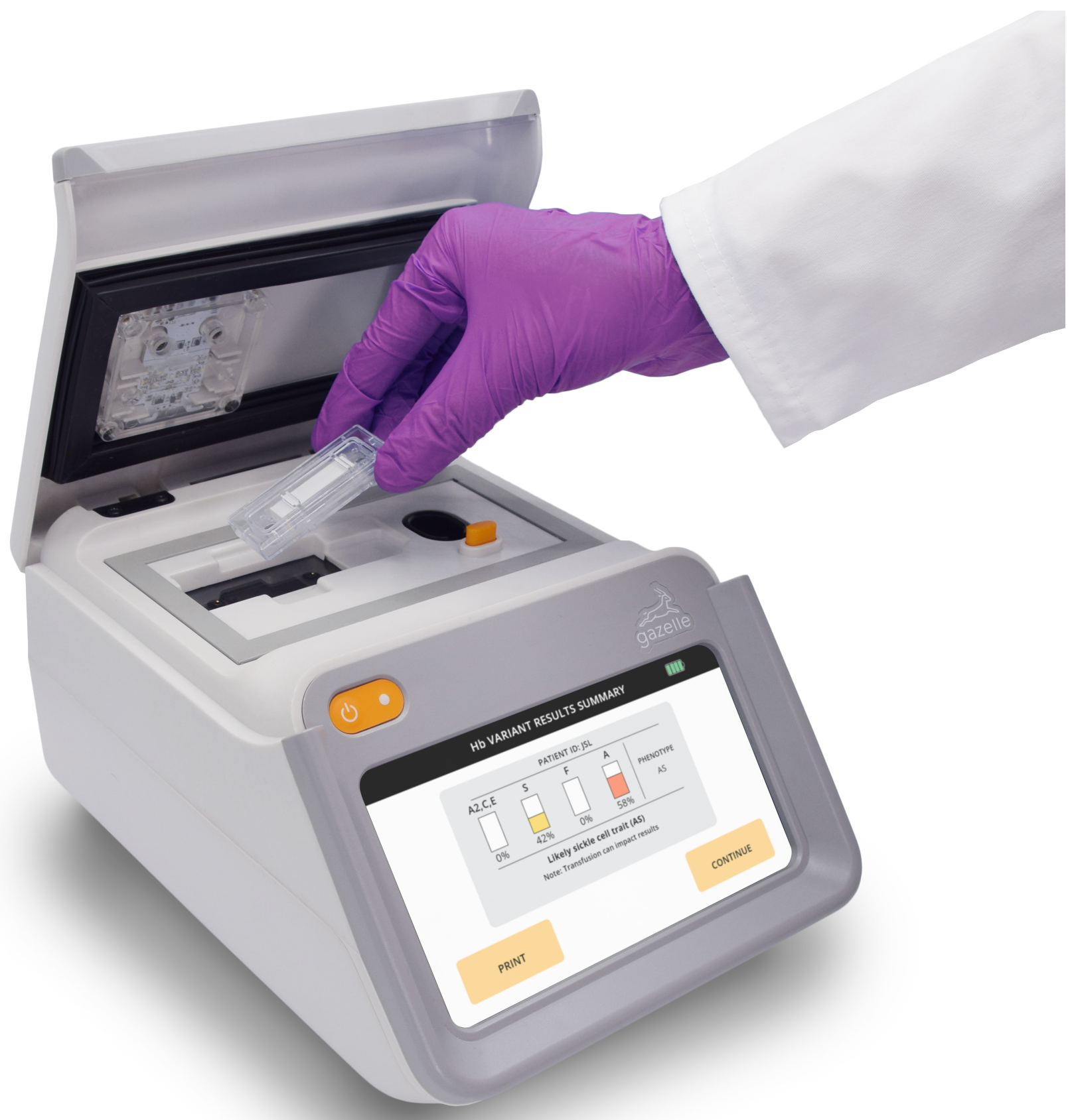
Figure 2. The rugged, lightweight, battery-powered Gazelle Diagnostic Device can withstand high temperatures and humidity. No cold chain management is required.
